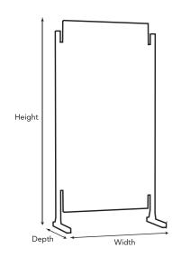
Dimensions: Height: 1835mm Width: 940mm Depth:: 410mm
