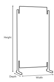
Dimensions: Height: 1175mm Width: 660mm Depth:: 200mm
